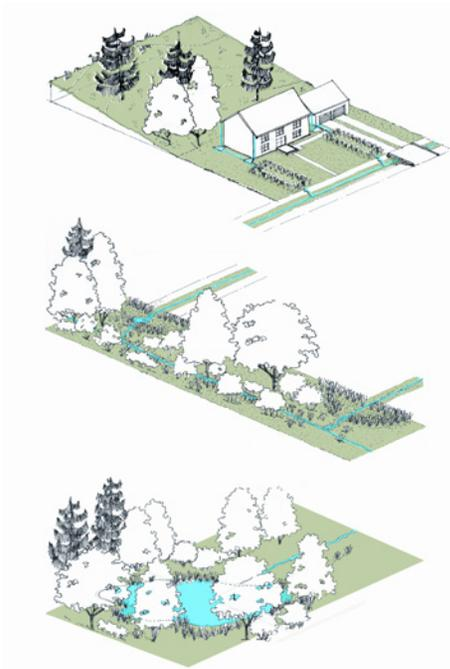
Figure 8: A treatment train includes multiple BMPs that convey, treat, and discharge rainwater.
